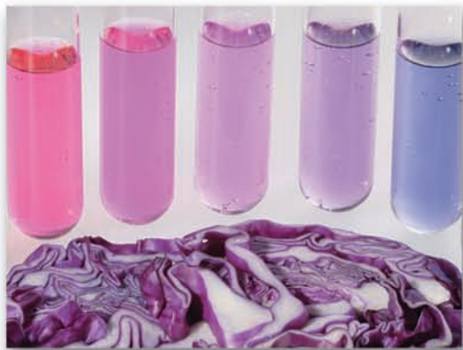
Natural Indicators Substances in red cabbage and other natural sources change color in acids and bases.
