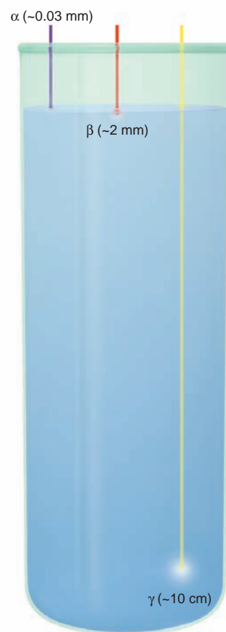
FIGURE 23.7 Penetrating power of radioactive emissions. Penetrating power is often measured in terms of the depth of water that stops 50% of the incoming radiation. (Water is the main component of living tissue.) Alpha particles, with the highest mass and charge, have the lowest penetrating power, and \gamma rays have the highest. (Average values of actual penetrating distances are shown.)
