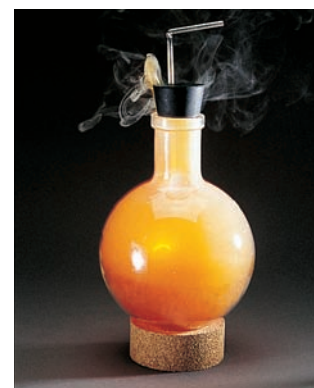
FIGURE 9.6 The reaction between sodium and bromine. A , Despite the endothermic electron-transfer process, all the Group 1A(1) metals react exothermically with any of the Group 7A(17) nonmetals to form solid alkali-metal halides. The reactants in the example shown are sodium (in beaker under mineral oil) and bromine. B , The reaction is usually rapid and vigorous.
