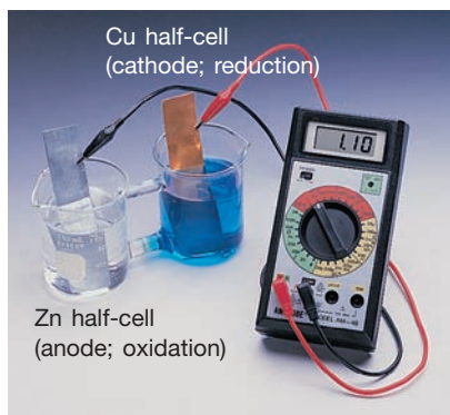
FIGURE 21.7 Measurement of a standard cell potential. The zinc-copper cell, operating at 298 K under standard-state conditions, produces a voltage of 1.10 V.
