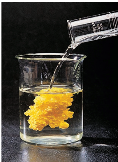
FIGURE 4.6 The reaction of Pb(NO 3 ) 2 and NaI. When aqueous solutions of these ionic compounds are mixed, the yellow solid PbI 2 forms.
