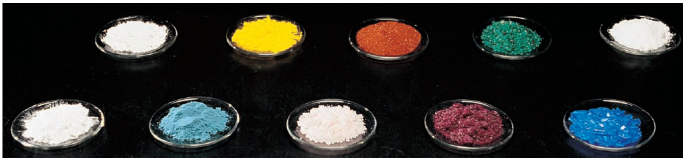
FIGURE 22.6 Colors of representative compounds of the Period 4 transition metals. Staggered from left to right, the compounds are scandium oxide (white), titanium(IV) oxide (white), vanadyl sulfate dihydrate (light blue), sodium chromate (yellow), manganese(II) chloride tetrahydrate (light pink), potassium ferricyanide (red-orange), cobalt(II) chloride hexahydrate (violet), nickel(II) nitrate hexahydrate (green), copper(II) sulfate pentahydrate (blue), and zinc sulfate heptahydrate (white).
