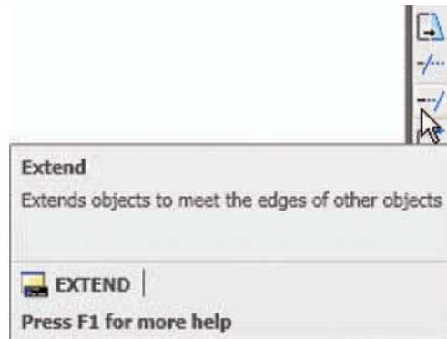
Fig. 5.39 The Extend tool icon in the Modify toolbar in the AutoCAD Classic workspace
