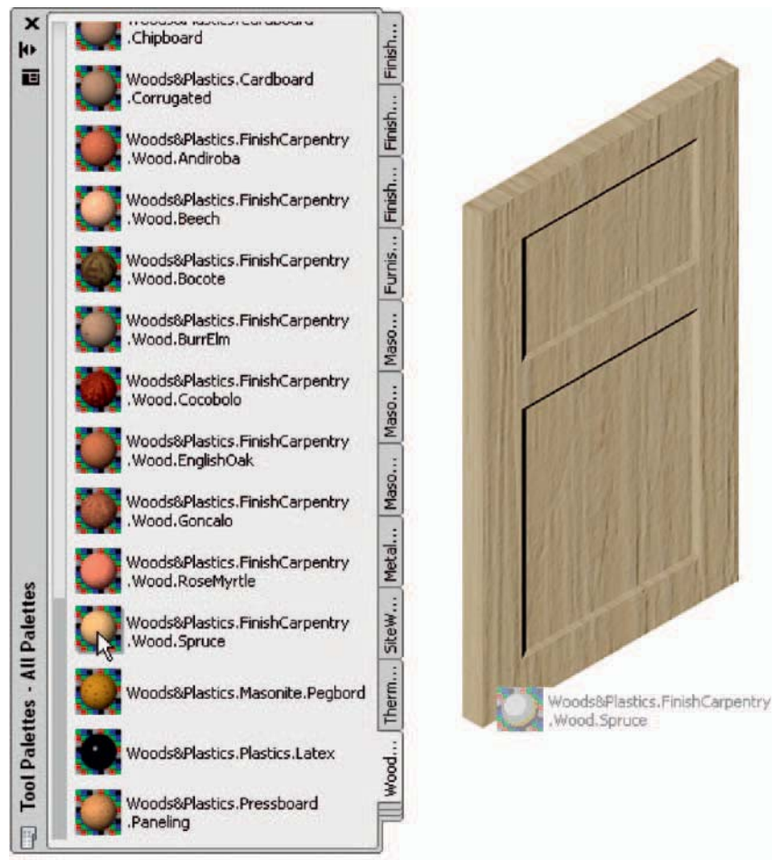
Fig. 15.14 Third example – applying a wood material
