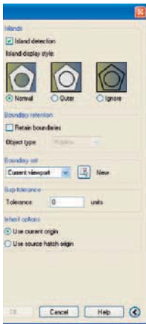
Fig. 8.11 The Island display style selections in the expanded Hatch and Gradient dialog
