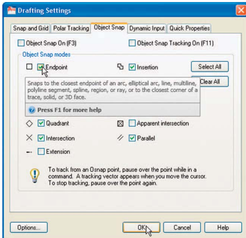
Fig. 3.12 The Drafting Settings dialog with some of the Object Snaps set on
