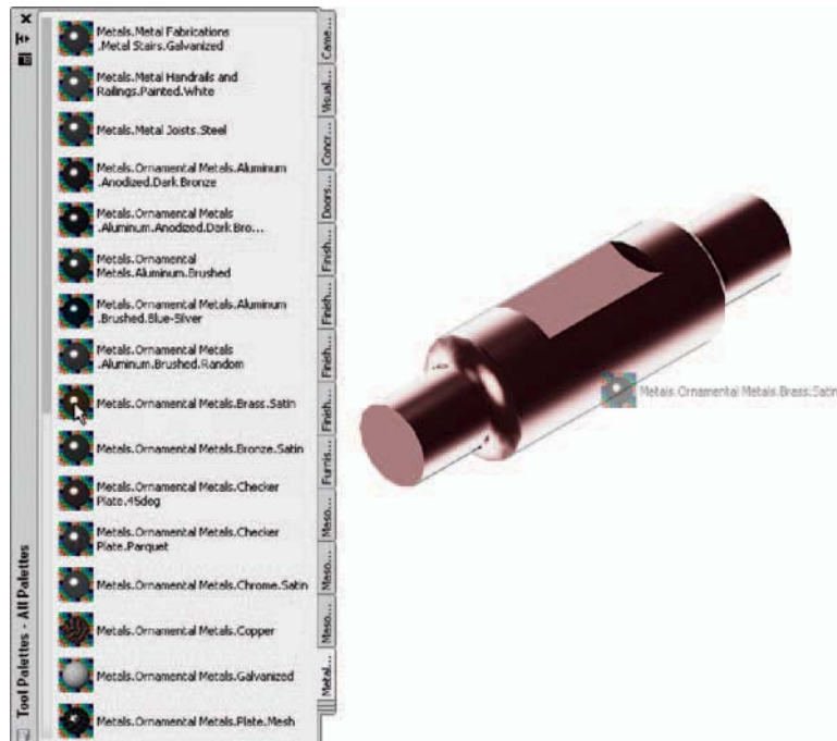
Fig. 15.13 Second example – applying a metal material
