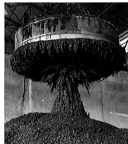
Fig. 28-1 Using an electromagnet to collect and transport scrap metal at a steel mill. (Digital Vision/Getty Images)
