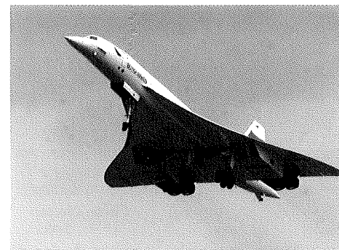
Fig. 18-9 When a Concorde flew faster than the speed of sound, thermal expansion due to the rubbing by passing air increased the aircraft's length by about 12.5 cm. (The temperature increased to about 128^\circ\text{C} at the aircraft nose and about 90^\circ\text{C} at the tail, and cabin windows were noticeably warm to the touch.) (Hugh Thomas/BWP Media/Getty Images News and Sport Services)
