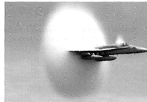
Fig. 17-23 Shock waves produced by the wings of a Navy FA 18 jet. The shock waves are visible because the sudden decrease in air pressure in them caused water molecules in the air to condense, forming a fog. (U.S. Navy photo by Ensign John Gay)
