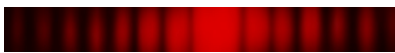
v / Single-slit diffraction of red light. Note the double width of the central maximum.
