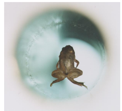
h / A frog is levitated diamagnetically inside a powerful magnet. Evidently frog has \mu < \mu_0 .
