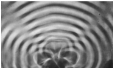
w / A pretty good simulation of the single-slit pattern of figure u, made by using three motors to produce overlapping ripples from three neighboring points in the water.
