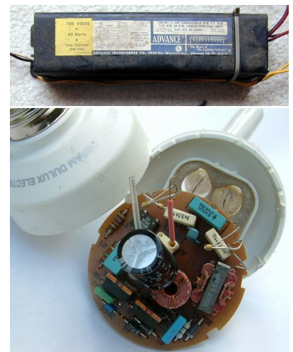
n / Ballasts for fluorescent lights. Top: a big, heavy inductor used as a ballast in an old-fashioned fluorescent bulb. Bottom: a small solid-state ballast, built into the base of a modern compact fluorescent bulb.
