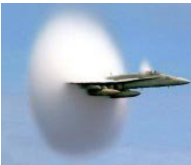
ab / This fighter jet has just accelerated past the speed of sound. The sudden decompression of the air causes water droplets to condense, forming a cloud.
